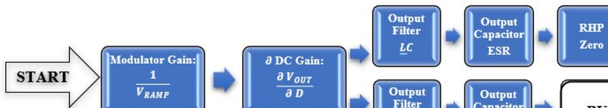
Figure 3.1: Intuitive diagram to identify all elements involved into the control to output TF evaluation for basic topologies (Right Half Plane zero included). Voltage mode CCM assumed.
